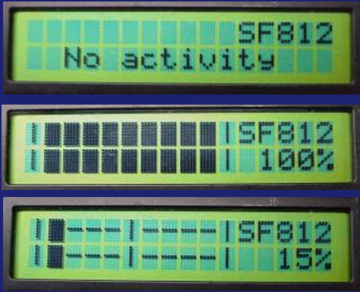
Pictured to the left is an example of the thermistor based measurement equipment. Above are examples of the gauge readout that would be seen by the divers during operations. 2
